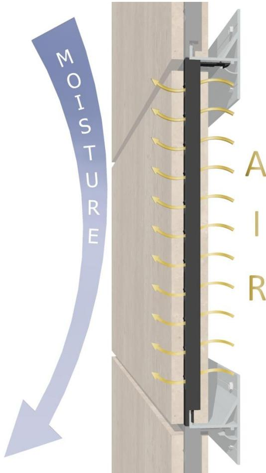
With cavity wall systems, the difference in air pressures across the exterior cladding is a significant force causing infiltration of air and water. As thunderstorms approach the air pressure in the cavity becomes less than the external air pressure along the building face. The natural equalization of this differential in air pressure causes the wall cavity to literally draw water into it.
