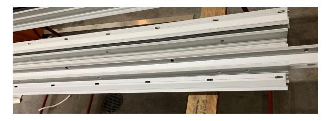
3. Set the bottom of the "Bottom J", or starter rail, on the mark and check your level again. Temporarily attach the rail using small needle-nose vise clamps. Now you can fasten the bottom Jay to the face of the mullions using the 1 ½" screws provided.
