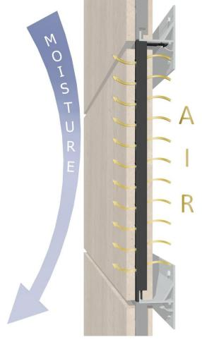
With cavity wall systems, the difference in air pressures across the exterior cladding is a significant force causing infiltration of air and water. As thunderstorms approach the air pressure in the cavity becomes less than the external air pressure along the building face. The natural equalization of this differential in air pressure causes the wall cavity to literally draw water into it.
