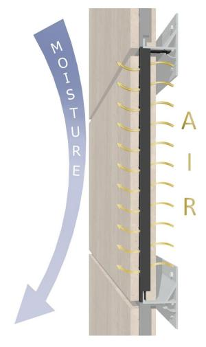
With cavity wall systems, the difference in air pressures across the exterior cladding is a significant force causing infiltration of air and water. As thunderstorms approach the air pressure in the cavity becomes less than the external air pressure along the building face. The natural equalization of this differential in air pressure causes the wall cavity to literally draw water into it.
